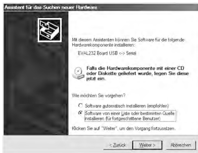
Figure 12-43. Installing the USB interface driver - 2 4. Select the data CD as the source.
